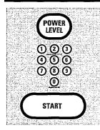
How to Change the Power Level The power level may be entered or changed immediately after entering the feature time for TIME COOK, TIME DEFROST or MINUTE COOK. The power level may also be changed during time countdown. **1** Press TIME COOK or select Time Defrost. 2 Enter cooking or defrosting time. **3** Press POWER LEVEL. 4 Select desired power level 1-10. 5 Press START.
